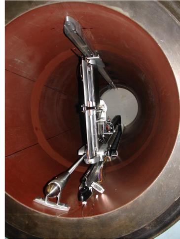
Figure 22. Three-dimensional traverse mounted in the test section of the HRTF. Jimenez (2007)
