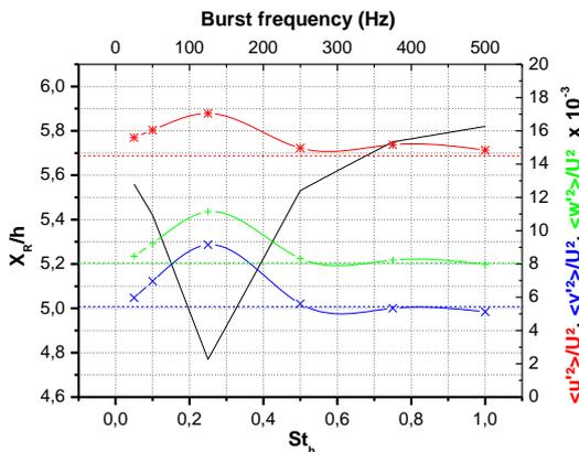
Figure 4. Normal Reynolds Stress component for unforced (dash lines) and forced case at several  $f_{BM}$  (solid lines).
