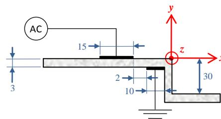
Figure 2. Sketch of the DBD actuator on the step, units in mm.
