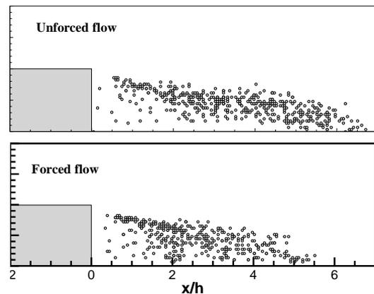
Figure 8. Vortex centres obtained by  $\Gamma_2$  criterion for 250 instantaneous fields.
