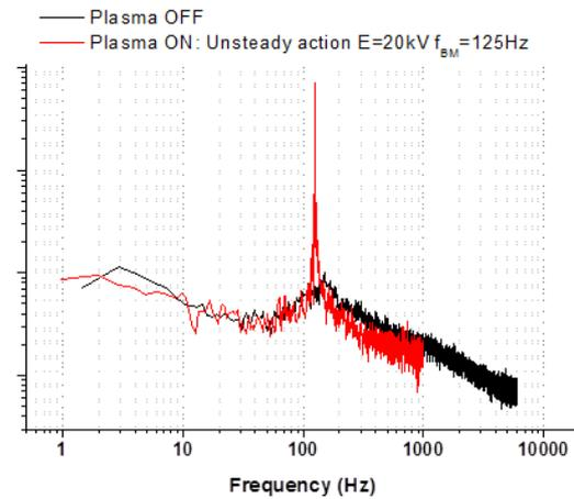
Figure 70. Spectre from LDV data ( $x/h=2$   $y=5$ mm).
