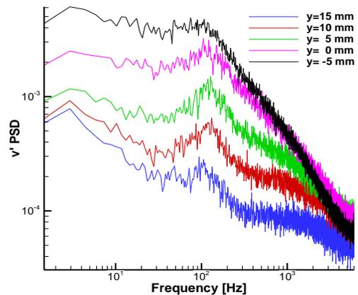
Figure 5. Local spectrum through the shear layer calculated by LDV for several positions in  $y$  ( $x/h=3$ ).
