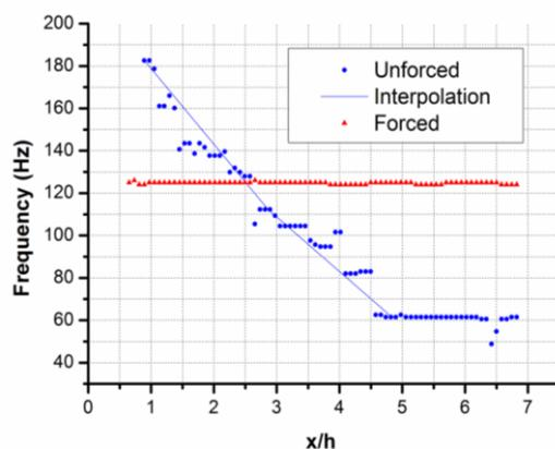
Figure 9. Evolution of the frequency with the distance downstream  $x/h$
