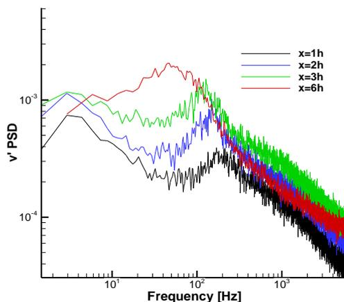
Figure 6. Local spectrum along the shear layer calculated for several positions  $x/h$  by LDV ( $y=5$  mm).
