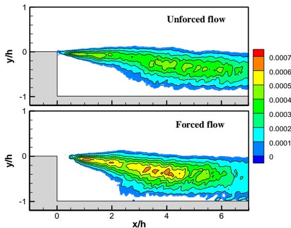
Figure 9. Production of TKE for unforced and forced flow.
