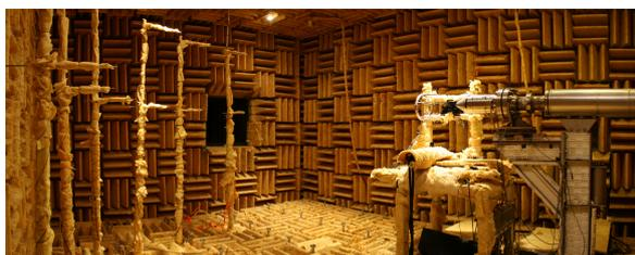
Figure 1. Syracuse University Anechoic Chamber
