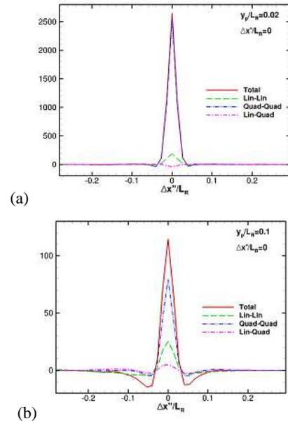
Figure 5 : Longitudinal profiles of the contributions to  $\langle p^2(\mathbf{x}) \rangle$  at the reattachment with  $\mathbf{x}' = (L_R, 0.02L_R, 0)$  - fig. 5a - and  $\mathbf{x}' = (L_R, 0.1L_R, 0)$  - fig. 5b - respectively.
