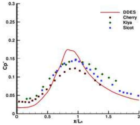
Figure 4 : Predicted  $C_p'$  versus experimental data
