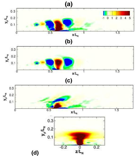
Figure 8 : Distributions of  $D_{\mathbf{x}}(\mathbf{x}')$  (a),  $D_{\mathbf{x}}^L(\mathbf{x}')$  (b) and  $D_{\mathbf{x}}^Q(\mathbf{x}')$  (c) in a longitudinal vertical plane for  $x=0.6L_R$ . (d) distribution of  $D_{\mathbf{x}}(\mathbf{x}')$  in the spanwise vertical plane for  $x=L_R$ .
