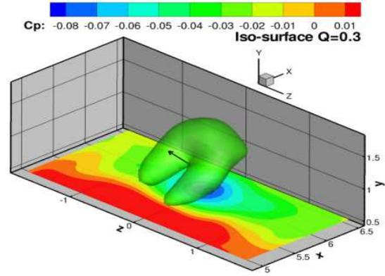
Figure 10 : Conditional Q and wall fluctuating pressure iso-surfaces. The condition for an event of second quadrant is  $u.v < -u_{rms}v_{rms}$  at  $x/L_R = 1$  and  $y/L_R = 0.1$  (maximum shear).
