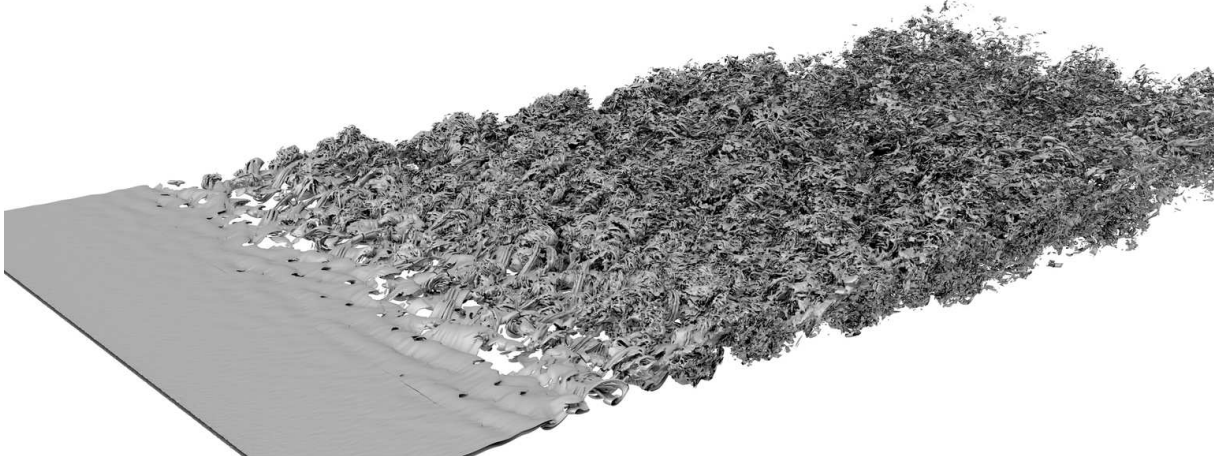
Figure 1. Isosurface of the vorticity magnitude. The whole domain is shown.
