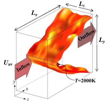
Figure 1. Computational configuration of DNS of turbulent V-shape premixed flame.
