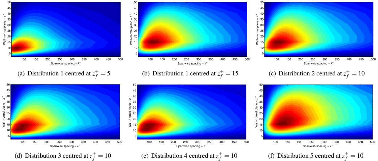
Figure 2. Response maps for  $\max_t(\mu)$  for fields (a)  $F_{1,x}$  at  $z_f^+ = 5$ , (b)  $F_{1,x}$  at  $z_f^+ = 15$ , (c)  $F_{2,x}$  at  $z_f^+ = 10$ , (d)  $F_{3,x}$  at  $z_f^+ = 10$ , (e)  $F_{4,x}$  at  $z_f^+ = 10$ , and (f)  $F_{5,x}$  at  $z_f^+ = 10$
