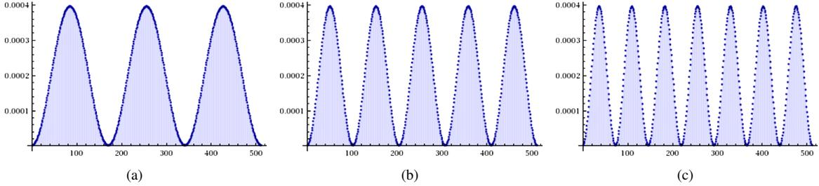
Figure 4. Wall-normal spectras using DST-I with 512 points for  $F_{1,x}$  located at (a)  $z_f^+ = 5$ , (b)  $z_f^+ = 10$  and (c)  $z_f^+ = 15$
