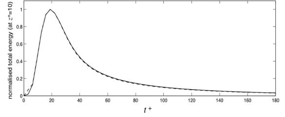
Figure 5. The impulse response: normalised time evolution of  $\mu$  evaluated at  $z^+ = 10$  for impulse initial conditions. Solid line:  $z_f^+ = 1.0$ ; Dashed line:  $z_f^+ = 0.5$ .
