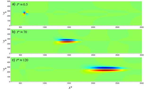
Figure 6. Plan view contours (taken at  $z^+ = 10$ ) of streamwise velocity perturbation at times (a)  $t^+ \approx 0.5$ , (b)  $t^+ \approx 70$  and (c)  $t^+ \approx 120$ .
