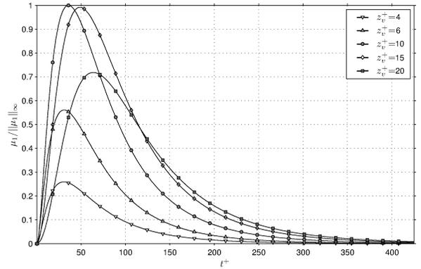
Figure 1. Transient growth of streamwise kinetic energy at different wall-normal locations  $z_v^+$  for body force at  $z_f^+ = 10$  and  $\lambda^+ = 100$ . Plots have been normalised using the global maximum.
