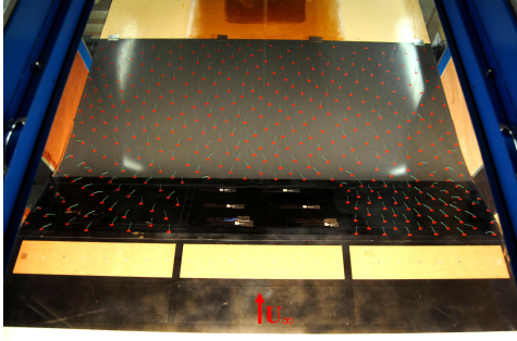
Figure 4. Example of wool tufts visualisation with control and no separation, \alpha = -2^\circ , \beta = -22^\circ and U_\infty = 10 m/s.
