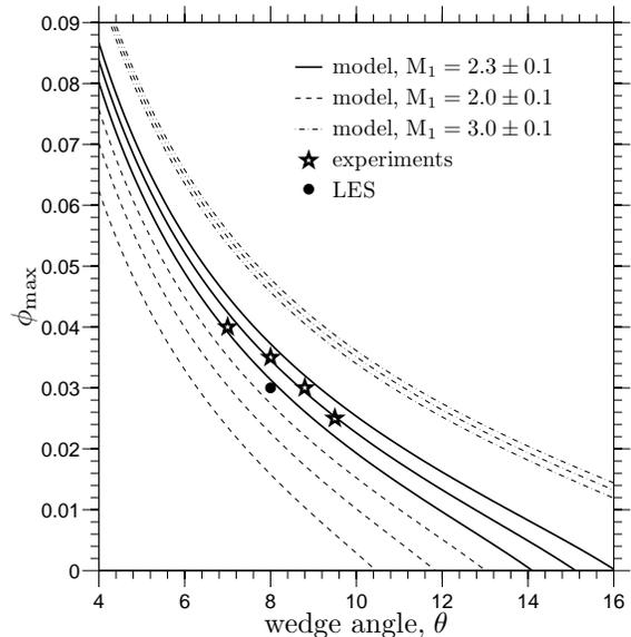
Figure 3: Predicted Strouhal-number value  $\phi_{\max} \equiv f_{\max}L/\bar{u}_1$  of the most energetic shock oscillations (at frequency  $f_{\max}$ ) for different upstream Mach numbers  $M_1$  and wedge angles  $\theta$ . Experimental and LES data are from Dupont et al. (2006) and Touber and Sandham (2009), respectively. For all cases, a variation of  $\pm 0.1$  in the upstream Mach number value is applied. Upstream skin-friction levels are the same as in Dupont et al. (2006)
