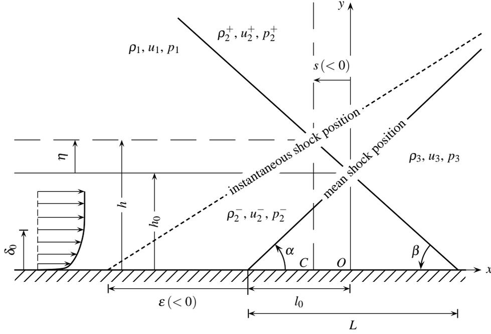
Figure 1: Sketch of the interaction with the definition of the notations in use
