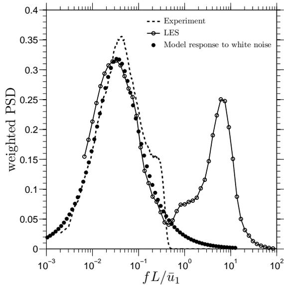
Figure 2: Premultiplied wall-pressure power-spectral-density distributions at the reflected-shock foot: model, large-eddy simulation (LES) and experimental results. The LES spectrum is taken from figure 17 in Touber and Sandham (2009) and the experimental data from Dupont et al. (2006)
