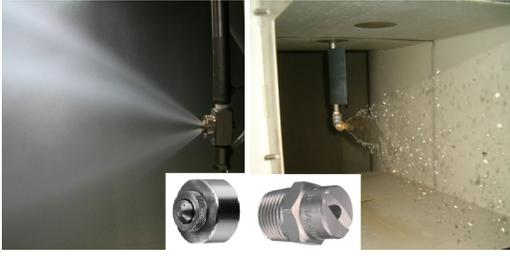
Figure 2. Close view of the spray heads and injected sprays (left: small droplets, Case 1; right: large droplets, Case 2).
