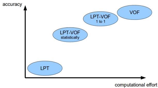
Figure 4. Qualitative comparisons of methods to simulate two-phase flows
