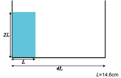
Figure 1. Initial state of water column in Koshizuka et al.'s (1995) experiment.
