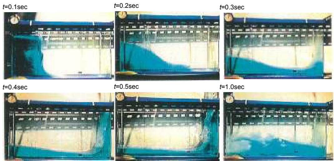
Figure 2. Experiments of Koshizuka et al. (1995) collapsing water column.
