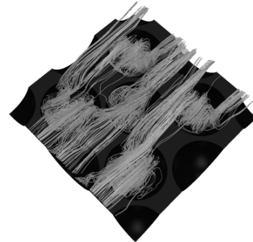
Figure 5: Time averaged streamlines at t^+ = 5 for dimple package with the depth to diameter ratio of t/D = 0.326 , Re_H = 13042 .
