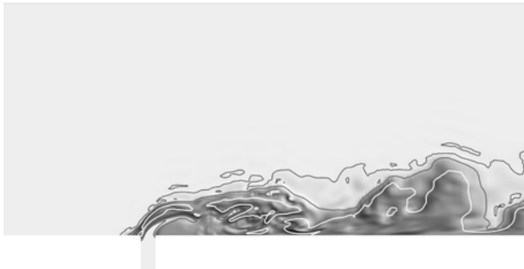
Figure 2. Mass fraction of water vapour. Black/white contour lines: Y_{H_2O} = 0.01 / 0.05
