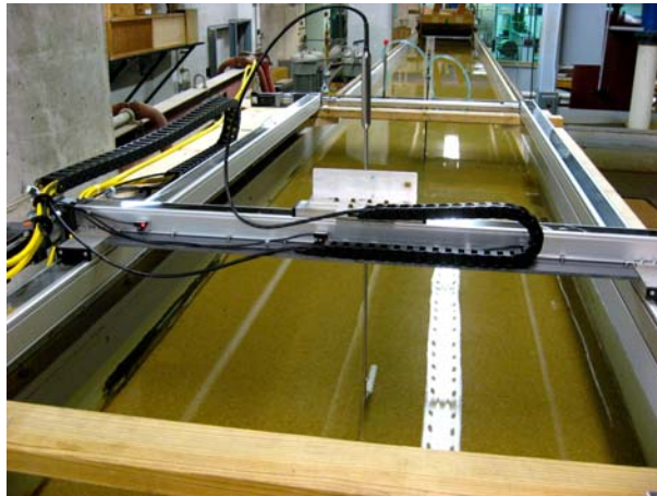
Figure 9. Photograph of the apparatus installed on the 24 m long tilting flume. The perspective is looking in the upstream direction. One conductivity sensor is installed for this example.
