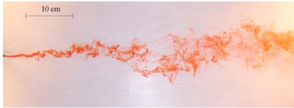
Figure 1. Flow visualization of the chemical plume, which is created via a continuous iso-kinetic release of a dye solution into a fully developed turbulent boundary layer. The view is from above, with the flow moving from left to right (Page et al. 2011a).
