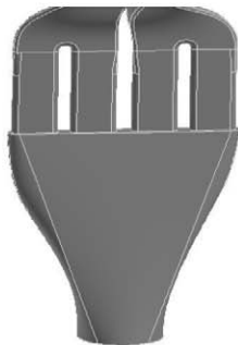
Figure 2: Picture showing the entrance manifold which changes from a circular pipe to the four large aspect ratio channels typically found in turbine blades.
