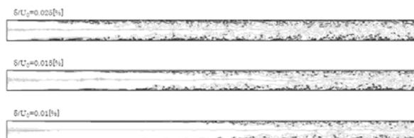
Fig. 5 Influence of inlet turbulence on the transition point. (Re=20,000. Grid points = 5,000×100×100. 4th-order Runge-Kutta scheme is used.  $(\sum_n \frac{\partial u_i}{\partial x_i} / N) \Delta x = \delta$ )
