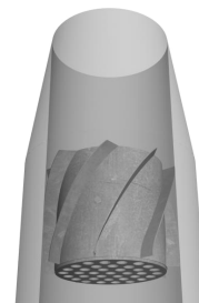
Figure 2: The perforated-plate/swirler-vanes configuration shown inside the burner nozzle.
