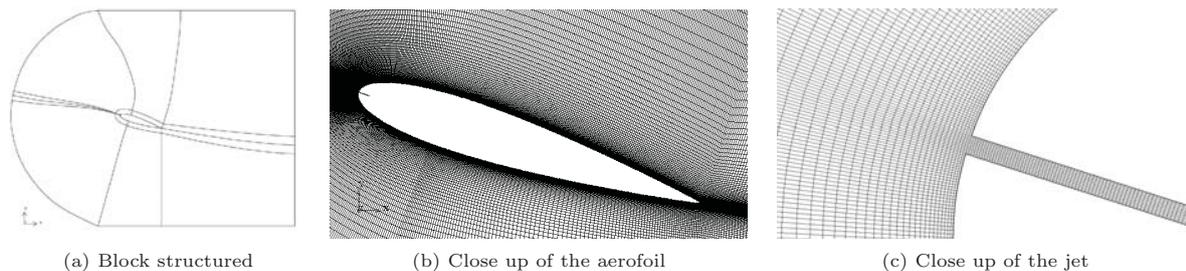
Figure 1: Structured mesh of 9.4M cells
