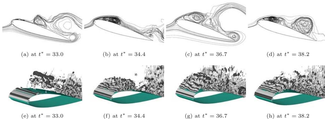
Figure 7: Instantaneous flow streamlines (*top*) and iso-surfaces of  $Q$  (*bottom*) from structured LES
