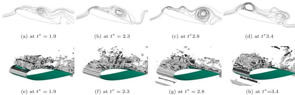
Figure 8: Instantaneous flow streamlines (*top*) and iso-surfaces of  $Q$  (*bottom*) from unstructured LES
