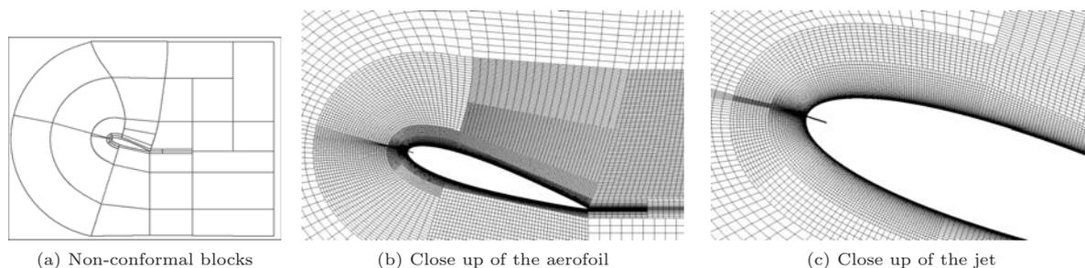
Figure 2: Unstructured mesh of 2M cells
