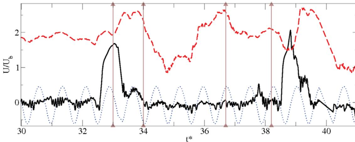
Figure 6: Time history of stream wise component of velocity at two locations; (*solid line*): close to leading edge ( $X_1, Y_2 = 0.1, 0.05$ ); (*dashed line*) close to mid-chord ( $X_2, Y_2 = 0.5, -0.06$ ); (*dotted line*): ZNMF jet velocity
