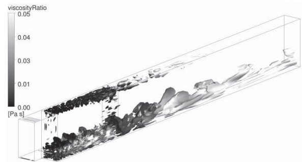
Figure 15. Backward facing step RANS (SAS). Viscosity ratio on isosurfaces of q -criterion (-2000).
