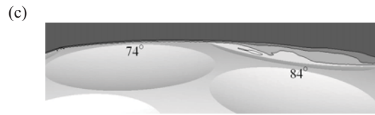
Figure 5 – Time-averaged contours of the streamwise velocity, Re = 1.1 \times 10^5 : (a) complete view (b) view at 52°, 63°; (c) view at 74°, 84° (angles measured from stagnation point at the front of the golf ball to the dimple centers)
