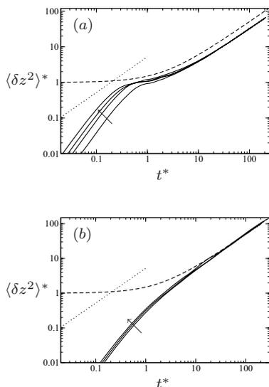
Figure 2: Time development of  $\langle \delta z^2 \rangle^*$  vs.  $t^*$ . The dashed and dotted lines show relations (3) and (4) respectively, and the solid lines DNS results. The arrow indicates the direction of decreasing  $F_h$  or increasing  $Re$ . (a) B-runs ( $\mathcal{R} \simeq 9$ ) and (b) D-runs ( $\mathcal{R} \simeq 6000$ ).
