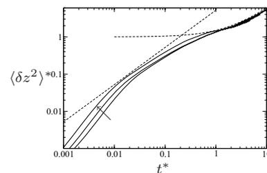
Figure 4: Time development of  $\langle \delta z^2 \rangle^*$ . The straight and bent thin dashed lines show relations (4) and (3) respectively. In both plots the solid lines show the result of the hyperviscosity simulations. The arrow indicates the direction of decreasing  $F_h$ .
