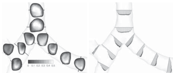
Figure 7: Velocity magnitude (left) and planar velocity profiles (right) in axis-normal slices of the human lung geometry.
