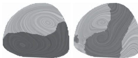
Figure 12: Line-integral-convolution and regions of positive (dark) and negative (light) helicity in an axis-normal slice close before second bifurcation of the human lung: extremal inspiratory (left) and expiratory condition (right).
