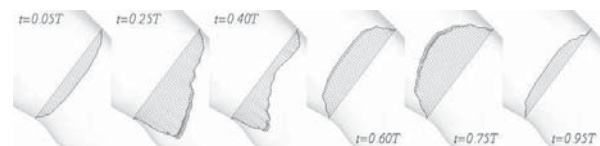
Figure 9: Velocity profiles in a central plane behind the first bifurcation of the human lung geometry for several stages in an oscillatory flow.
