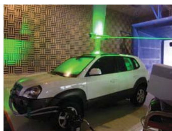
Fig. 3: PIV measurement of velocity fields over a sunroof opening in the test section of HAWT.
