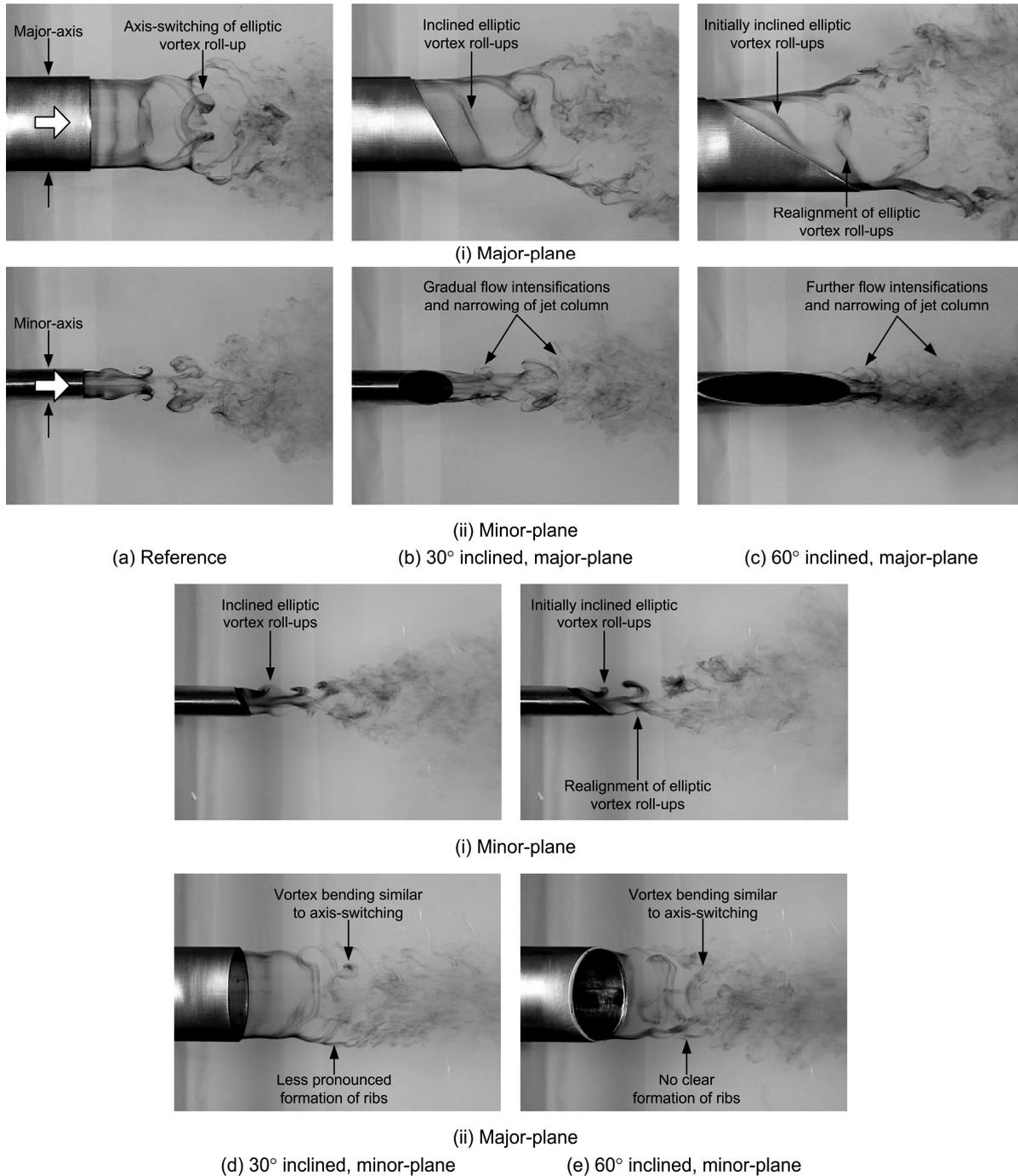
Fig. 2 Instantaneous flow visualization images for all inclined elliptic nozzles tested in the present study.
