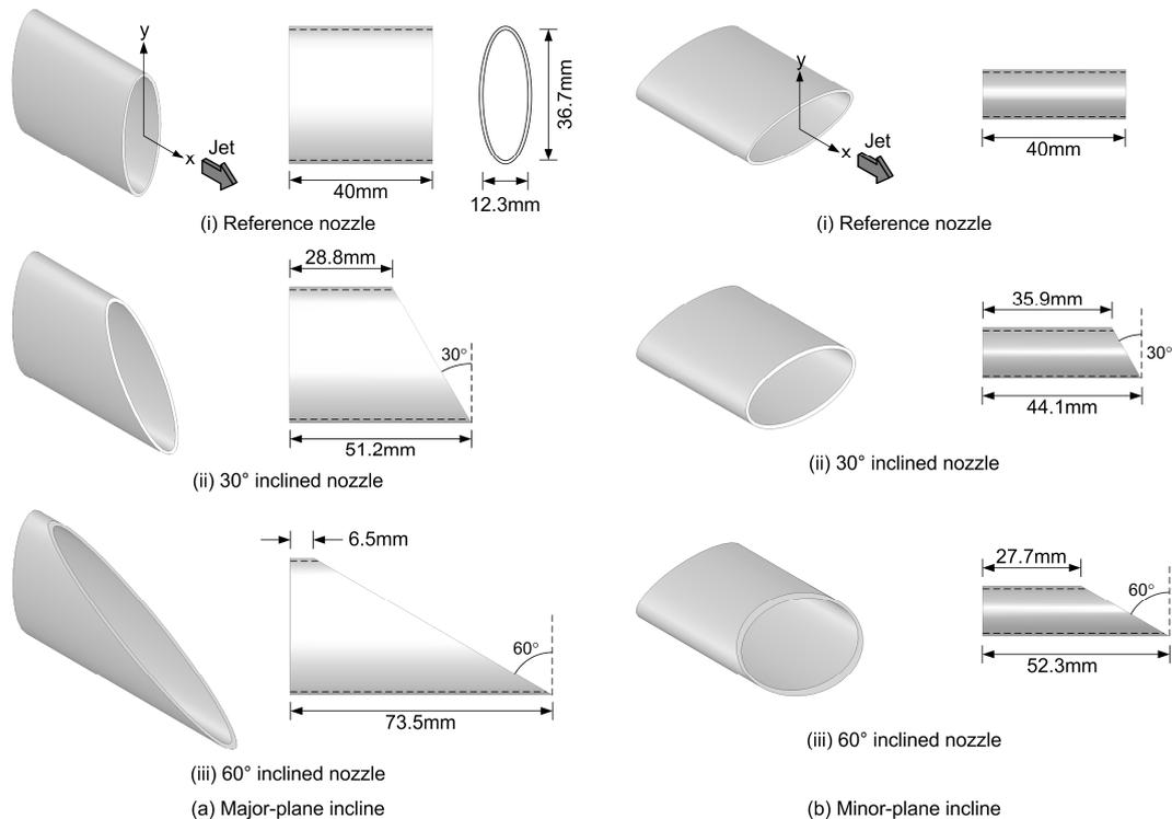
Fig. 1 Inclined elliptic nozzle designs used in the present study, which consist of inclines along the (a) major-plane and (b) minor-plane.
