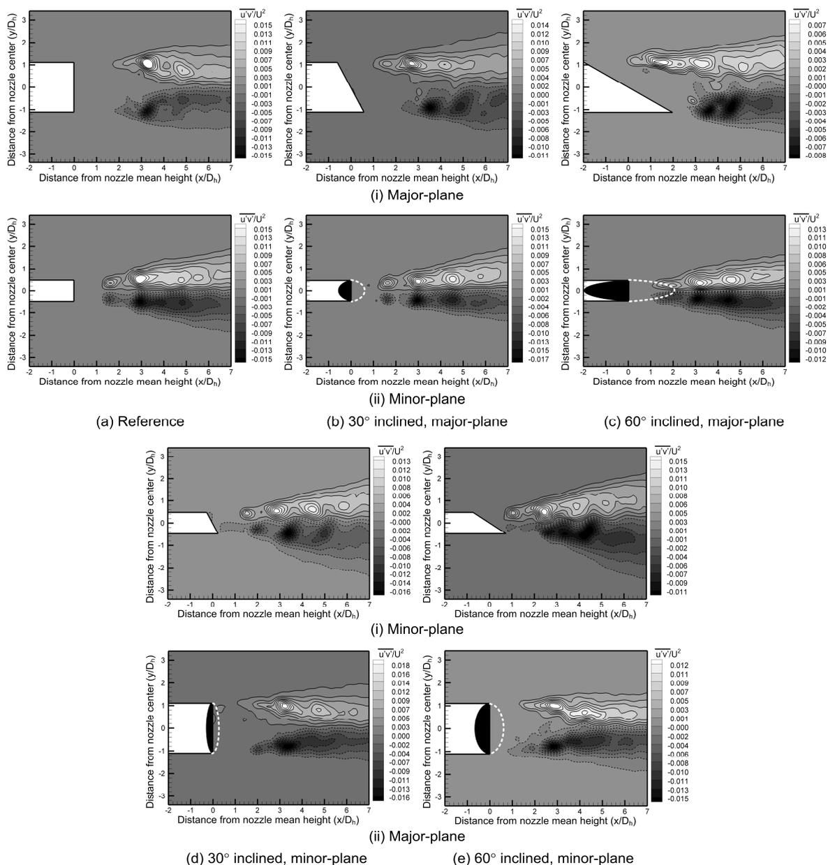
Fig. 4 Time-averaged Reynolds flow stress distributions for all inclined elliptic nozzles tested in the present study.
