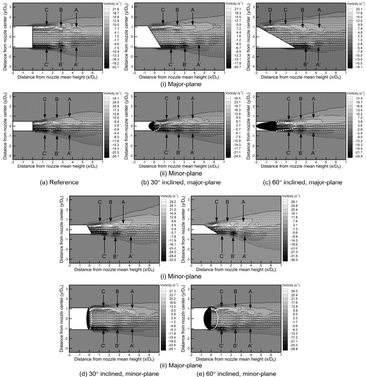
Fig. 3 Time-averaged vorticity field distributions for all inclined elliptic nozzles tested in the present study.
