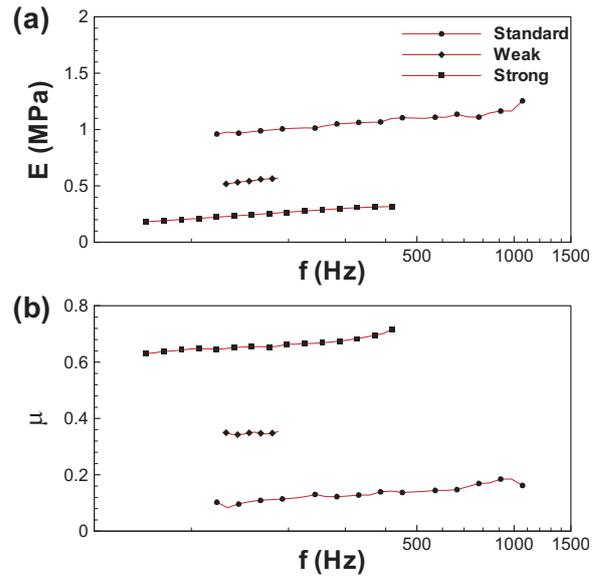
Fig. 2: Modulus of elasticity (a) and the loss tangent (b) vs. frequency.  $\blacktriangle$  - “standard”;  $\bullet$  - “weak”;  $+$  - “strong” compositions.
