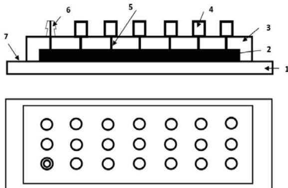
Fig. 1: The mould to prepare the compliant coating.
