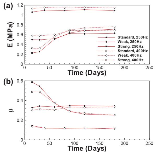
Fig. 3: Changing of the modulus of elasticity (a) and loss tangent (b) with time.
