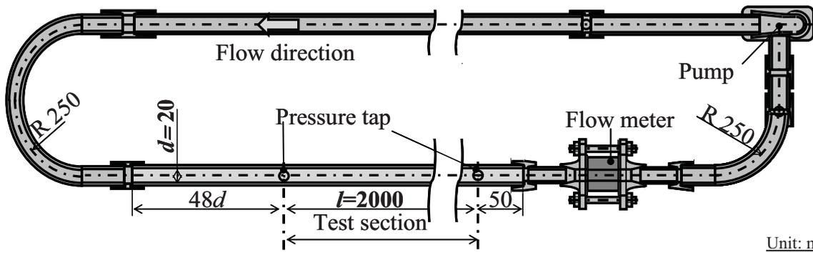
Fig. 1 Schematic of top-view experimental device.
