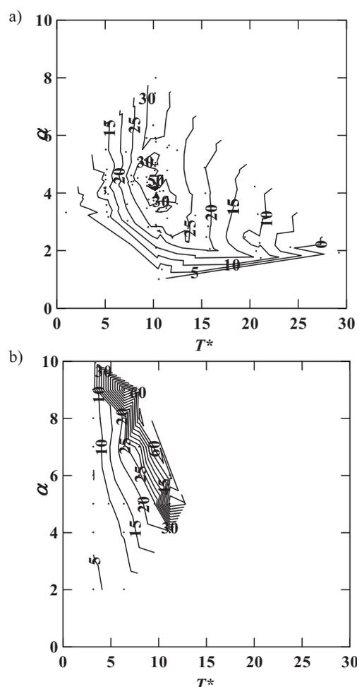
Fig. 4 Dependence of drag reduction rate upon pressure gradient in the acceleration period  $\alpha$  and cycle period  $T^*$  at  $Re_\tau=110$ ; (a) present results, (b) results from DNS by sasou *et al.* (2007). Each dat represents each datum point.
