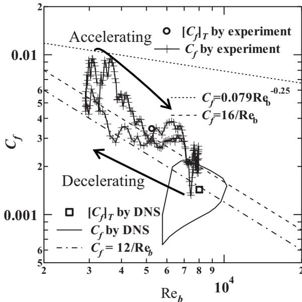
Fig. 6 Phase-averaged friction coefficient  $C_f$ . Present result at  $Re_\tau=110$ ,  $T^*=10$  and  $\alpha=4.1$ ; result from DNS by Sasou *et al.* (2007) at  $Re_\tau=110$ ,  $T^*=11.2$  and  $\alpha=5$ .
