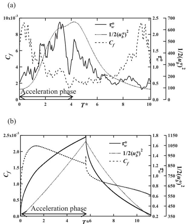
Fig. 7 Time trace of skin friction coefficient  $C_f$ , numerator  $\tau_w$  and denominator  $1/2(u_b^*)^2$  of Eq. (6). (a) present result at  $Re_\tau=110$ ,  $T^*=10$  and  $\alpha=4.1$ ; (b) DNS result at  $Re_\tau=110$ ,  $T^*=11.2$  and  $\alpha=5$  by Sasou *et al.* (2007)
