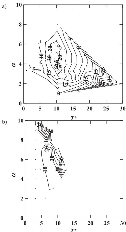
Fig. 3 Dependence of energy saving rate at the energy recovery rate of 100% for the negative pressure gradient phase upon pressure gradient in the acceleration period  $\alpha$  and cycle period  $T^*$  at  $Re_\tau=110$ ; (a) present results, (b) results from DNS by sasou *et al.* (2007). Each dat represents each datum point.
