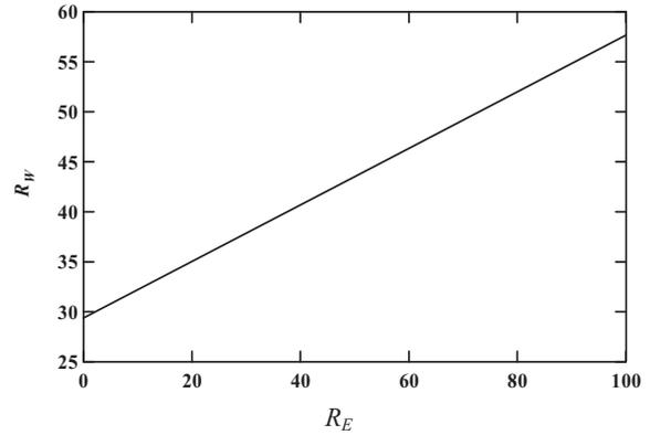
Fig. 9 Energy saving rate  $R_W$  versus energy recovery rate  $R_E$  at  $Re_\tau=110$ ,  $T^*=10$  and  $\alpha=4.1$ .
