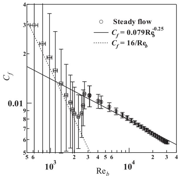
Fig. 2 Skin friction coefficient  $C_f$  for steady flow.
