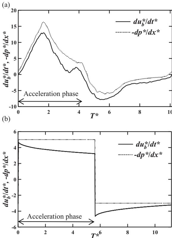
Fig. 8 Time trace each term on right-hand side of Eq (5). (a) present result at  $Re_\tau=110$ ,  $T^*=10$  and  $\alpha=4.1$ ; (b) DNS result at  $Re_\tau=110$ ,  $T^*=11.2$  and  $\alpha=5$  by Sasou *et al.* (2007)
