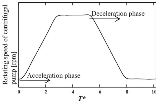
Fig. 5 Examples of time trace of rotating speed of centrifugal pump for best experimental condition.
