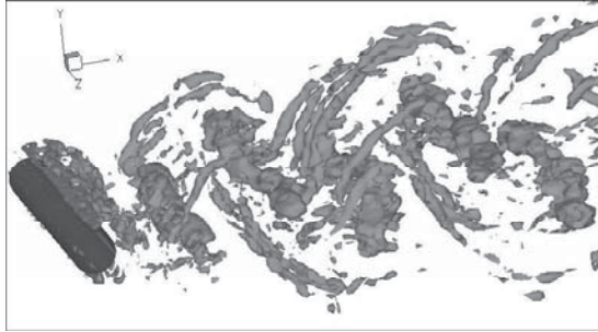
Figure 11: x-vorticity-isosurfaces \pm 1.5^{-1} s^{-2} of round cylinder at Re = 3,900 .
