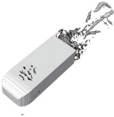
Figure 13: Iso-surface of instantaneous pressure fluctuation ( p'/\rho u_\infty^2 = -0.05 ).
