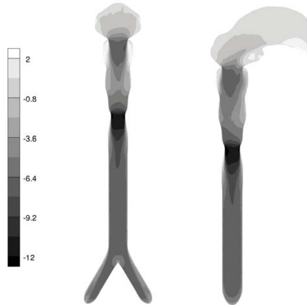
Figure 4: Isopleths of time-averaged velocity in the oral, pharyngeal, and tracheal regions along the tracheal axis.
