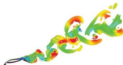
Figure 4: Illustration of resolved instantaneous vortex motion with the HYB0 model ( $\alpha = 25.2^\circ$ ).
