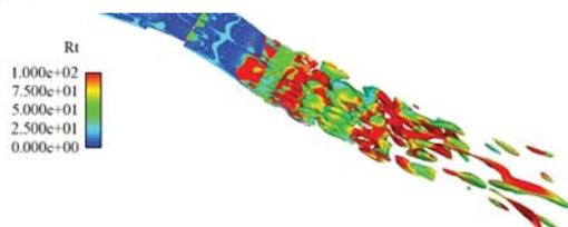
Figure 8: Resolved instantaneous vortex motion with the HYB0 model (with prescribed transition) at  $\alpha = 12.2^\circ$ .
