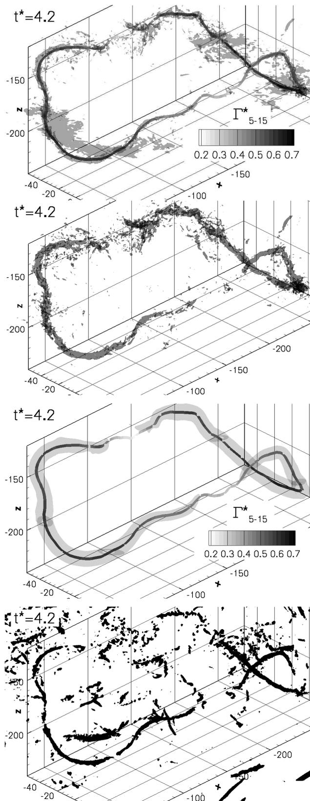
Figure 4: Iso-surfaces at  $t^* = 4.2$  for corrector criteria a) absolute vorticity  $|\vec{\omega}|$ , b)  $\lambda_2$ , c) pressure  $P$  and d) curvature  $i_\kappa$  cutout represents the x-values ranging from -100 to -200. The second peak is due to inflection points, where a straight line would be the best fit. However, the process checks radii
