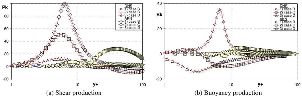
**Fig. 6 Production of turbulent kinetic energy**
