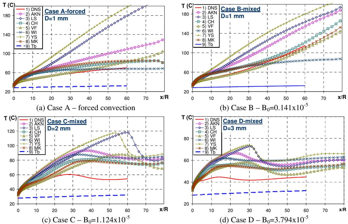
Fig. 1 Development of wall and bulk temperatures along the pipe
