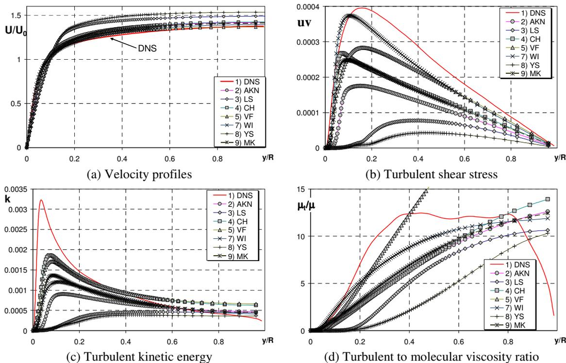
Fig. 3 Forced convection with flow acceleration due to heating (Case A)
