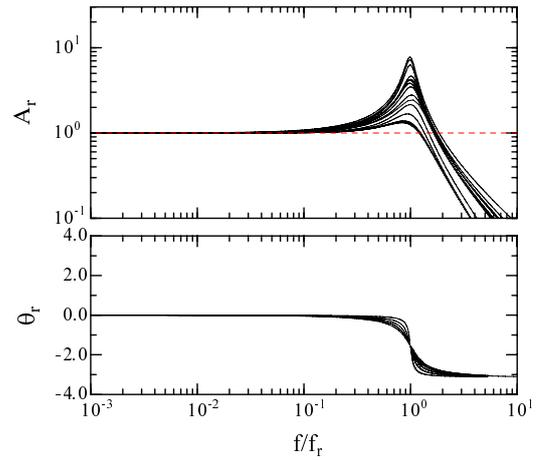
Figure 5: Helmholtz resonance generated inside pressure tube. Amplitude  $A_r$  and phase delay  $\theta_r$  are given in Eqs. (10) and (11).
