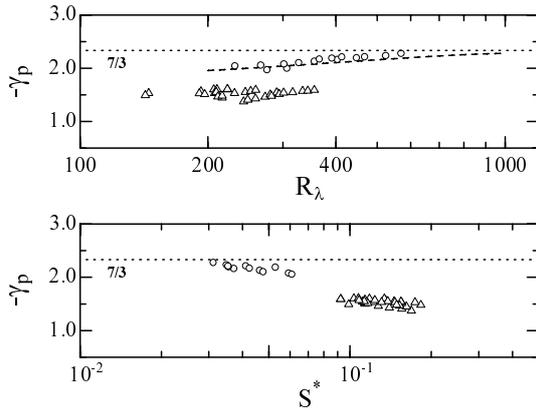
Figure 9: Scaling exponent of pressure spectra defined in Eq.(14) are plotted against Reynolds number and shear parameter.
