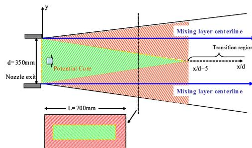
Figure 1: Driving mixing layer and coordinate system.
