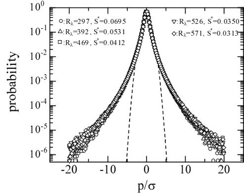
Figure 7: Probability density functions of pressure gradient measured in the mixing layer.
