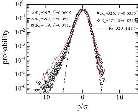
Figure 6: Probability density functions of pressure fluctuations measured in the mixing layer. The solid line is the case of no shear ( $dU/dy = 0$ ).
