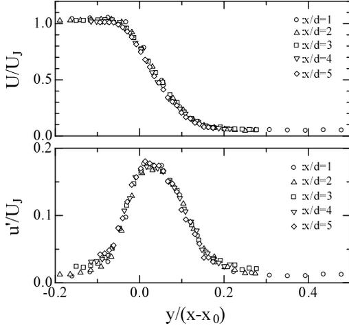
Figure 2: Mean and root mean square of stream-wise velocity component for the case of  $U_J = 6.0\text{m/s}$ . Different symbols indicate different  $x/d$  positions.
