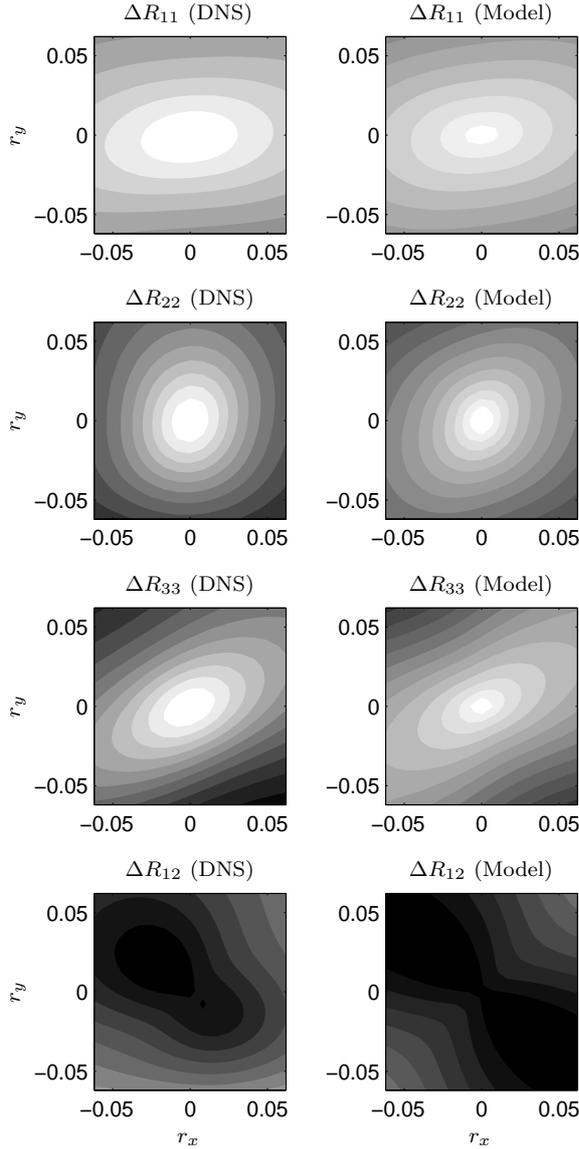
Figure 4: Isocontours of  $\Delta R_{ij}(y, \mathbf{r}) = R_{ij}(y, \mathbf{r}) - R_{ij}(y, 0)$  at  $y^+ = Re_\tau y/h = 114$ , plotted for  $r_z = 0$ . The correlations in the left column were calculated from DNS of channel flow, and the correlation in the right column from the best fit of the model with DNS. The contour levels for a given a correlation component (i.e. for the same row) have the same range.
