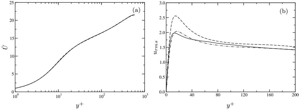
Figure 1: Mean and rms velocity profiles in wall coordinates from LES (—), DNS of Moser *et al.* (1999) (---) filtered DNS (· · ·). Shown are (a) mean velocity, (b) rms streamwise velocity  $u_{rms}$  in channel flow at  $Re_\tau = 590$ , with Fourier truncation filter widths of  $\Delta x^+ = 116$  and  $\Delta z^+ = 58$
