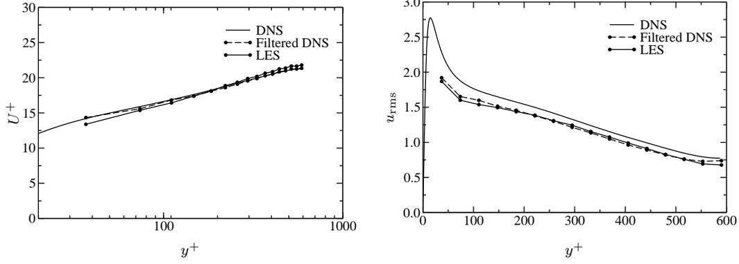
Figure 2: Mean velocity (left) and rms streamwise velocity fluctuations (right) in a turbulent channel at  $Re_\tau = 590$ . The LES was performed using the filtered boundary optimal LES formulation of Moser *et al.* (2007).
