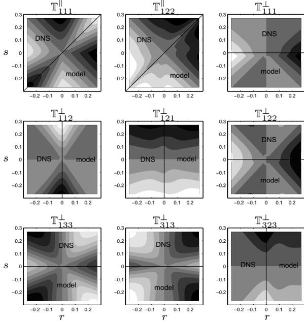
Figure 3: Contours of the DNS data of Langford and Moser (1999) and tensor model for  $\mathbf{r}$  and  $\mathbf{s}$  co-linear ( $\mathbb{T}^{\parallel}$ ) and orthogonal ( $\mathbb{T}^{\perp}$ ), in the  $r$ - $s$  plane. Each component has a symmetry, which is used to allow the data and the model to be displayed side-by-side, as shown. The heavy black lines are lines of symmetry for each component.
