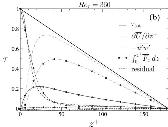
Figure 5: Individual shear-stress contributions for  $Re_\tau = 360$ , for unladen and laden flow ( $\phi_m = 0.65$ ,  $\tau_p^+ = 58$ );  $\bullet$ : laden.
