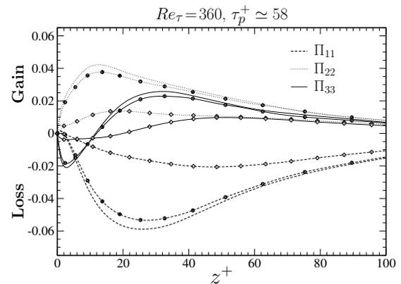
Figure 6: Effect of the mass-loading on the the re-distribution of energy term between the normal Reynolds-stresses ( $\Pi_{\alpha\alpha}$ ); —: unladen;  $\bullet$ :  $\phi_m = 0.16$ ;  $\diamond$ :  $\phi_m = 0.65$ .
