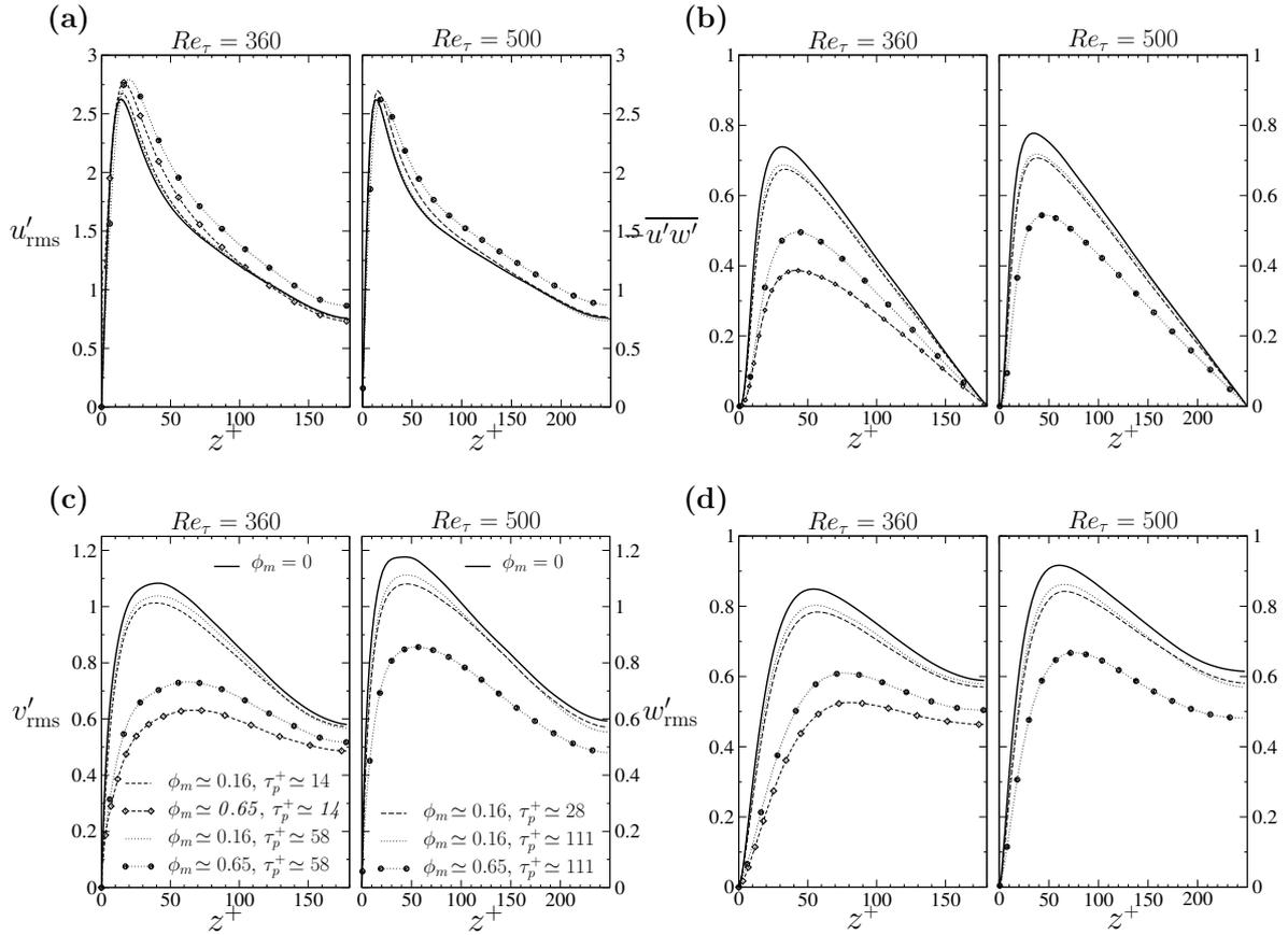
Figure 4: Turbulence intensity modification. (a) streamwise  $u'_{rms}$ , (b) shear-stress  $-\overline{u'w'}$ , (c) spanwise  $v'_{rms}$ , (d) normalwise  $w'_{rms}$ .
