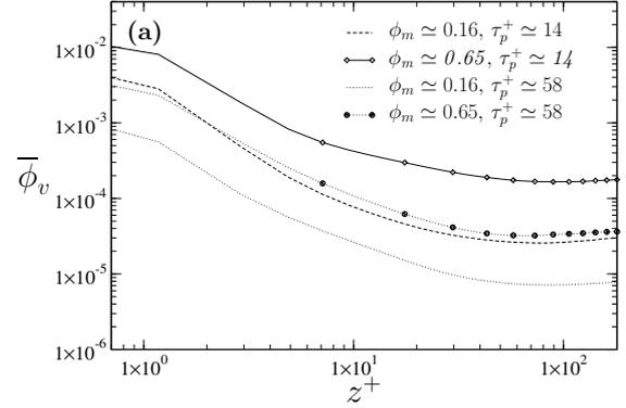
Figure 2: Concentration profile (volume-fraction of the dispersed phase,  $\bar{\phi}_v$ ) for  $Re_\tau = 360$ .
