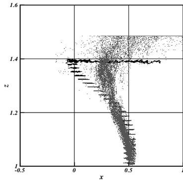
Figure 12: Side view of the plume at  $t = 1.1$ . Grey particles are Case  $Ri \rightarrow 0$ ; Black particles are Case  $Ri = 40$ .
