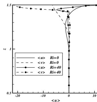
Figure 2: Vertical profile of the non dimensional mean horizontal velocity components.
