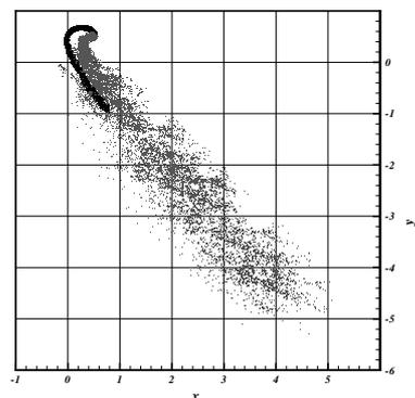
Figure 11: Top view of the plume at  $t = 1.1$ . Grey particles are Case  $Ri \rightarrow 0$ ; Black particles are Case  $Ri = 40$ .
