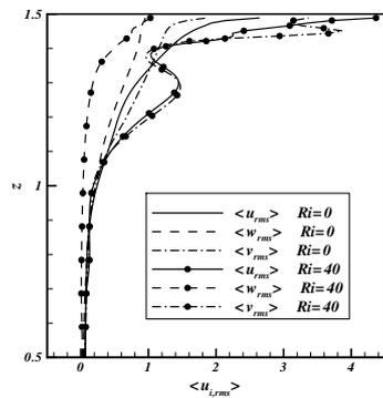
Figure 4: Vertical profile of the normal Reynolds stresses.
