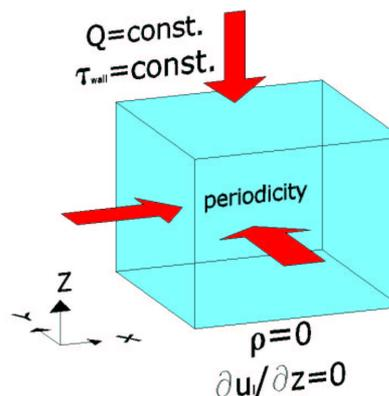
Figure 1: Schematic of the physical problem herein investigated. The quantity  $Q$  denotes the free surface heat flux.
