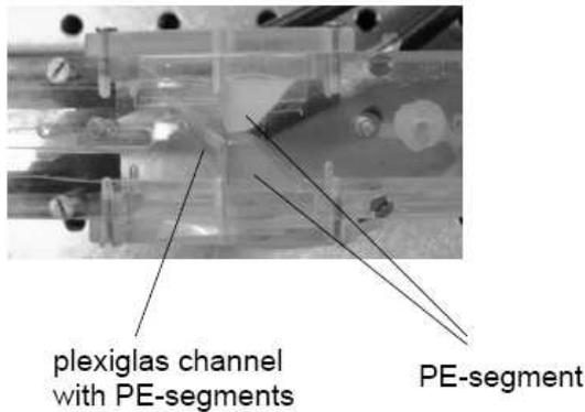
Figure 5: Measurements of vocal folds vibration by using Laser-Scanning-Vibrometer
