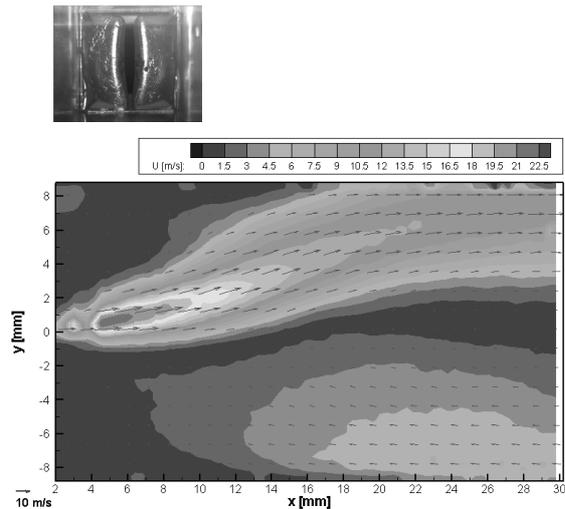
Figure 9: Vector plot and contour plot of the velocity downstream the vocal folds and the correspondent glottis opening stream of the vocal folds. This process is not tied to one specific vocal fold. Instead the sides are changed in a stochastic manner.
