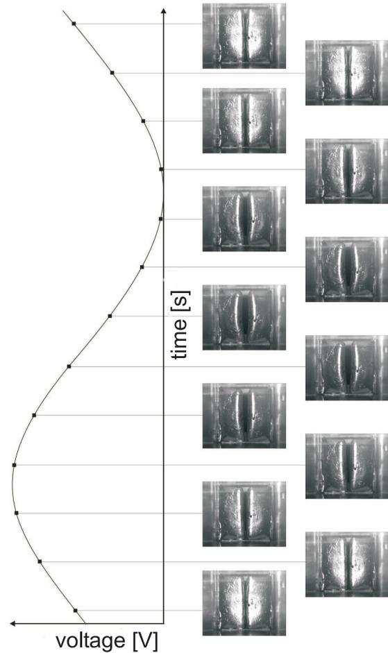
Figure 7: Form of the glottis during a whole oscillation cycle in reference to the pressure signal upstream the glottis
