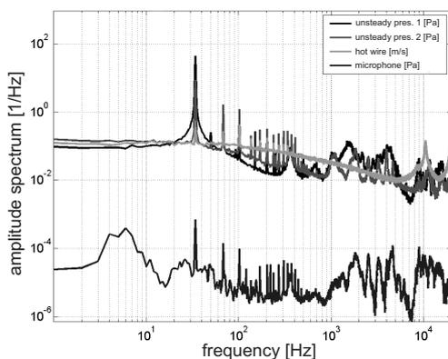
Figure 10: Amplitude spectrum of the unsteady pressure at two positions in the testsection, of the velocity measured by the Constant-Temperature-Anemometry and of the acoustic sound measured by the microphone
