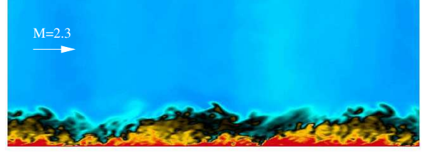
Figure 3: Instantaneous temperature field (boundary layer without incident shock).
