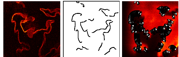
Figure 13: CH fluorescence image (left), detected flame front (center) and OH fluorescence image with unit vectors normal to the flame front (right).
