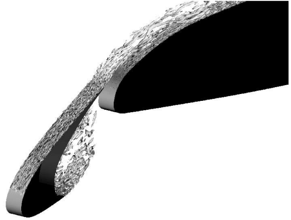
Figure 10: Turbulent structures in the slat area visualized by \lambda_2 contours with mapped on Mach number distribution.
