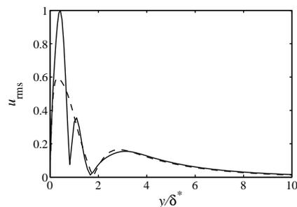
Figure 7: Waveforms of the — streaky TS-waves compared to the corresponding normal TS waves (---) at  $Re_x = 482000$ . The amplitude of the streaky waves are rescaled by 110 to account for the lower growth rate.
