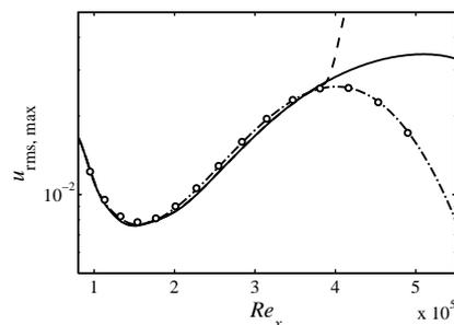
Figure 3: Comparison of TS-waves obtained by LES with LST and PSE. Wall-normal maximum of  $u_{\text{rms}}$  for --- uncontrolled case with random 3D disturbances, — 2D nonlinearly-saturated TS-wave, - · - linear low-amplitude TS-wave (rescaled), o PSE.
