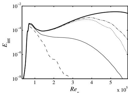
Figure 5: Energy integrated in the wall-normal direction contained in mode  $(\omega_0, 0)$  of the two-dimensional TS waves at  $F = 120$  in the presence of streaks. ---streak B, —streak C, .....streak E, -.-streak F, — no streak (case N).
