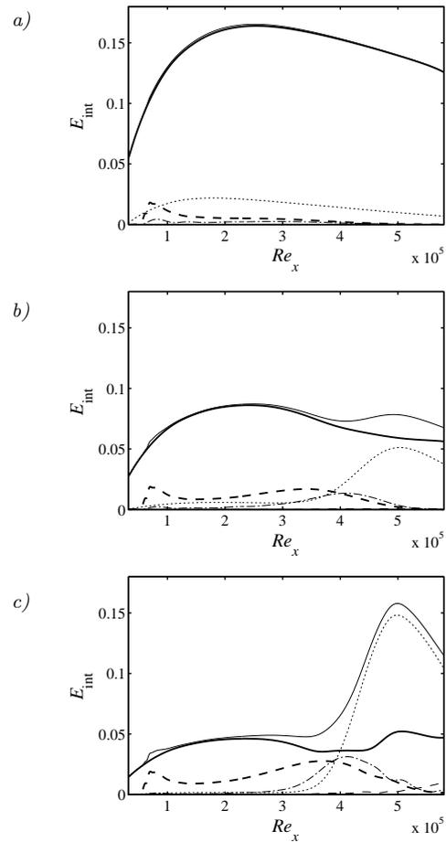
Figure 9: Energy integrated in the wall-normal direction for selected From a) to c): Streaks C, D, E, respectively. — Steady streak  $(0, \beta_{\text{st}})$ , - - - -TS-wave  $(\omega_0, 0)$ , ····· first harmonic of streak  $(0, 2\beta_{\text{st}})$ , - - - -first harmonic of streaky TS-wave  $(\omega_0, \beta_{\text{st}})$ , - - - -oblique mode  $(\omega_0, \beta_{\text{st}}/3)$ , — sum of all displayed modes.
