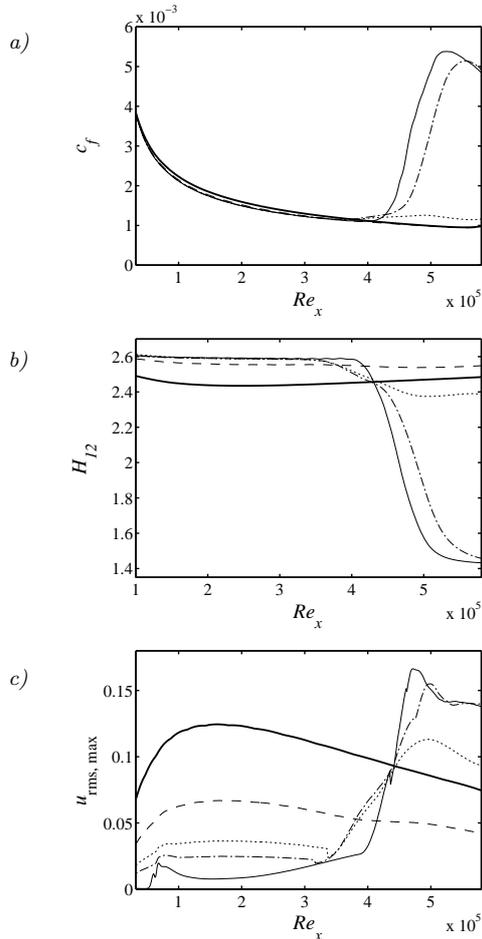
Figure 8: a) Skin friction coefficient  $c_f$ , b) shape factor  $H_{12}$ , and c)  $u_{\text{rms,max}}$  averaged in time and spanwise direction. — Streak C, - - - -streak D, ····· streak E, - - - -streak F, — case N (uncontrolled).
