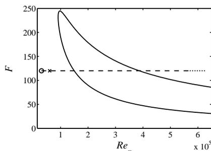
Figure 1: Stability diagram showing the neutral curve for two-dimensional TS waves. The dashed line signifies the computational domain with inlet at  $Re_x = 32000$  (o), and the cross  $\times$  indicates the streamwise position where the volume forcing is applied. The dotted line is the fringe region downstream of  $Re_x = 590000$ .
