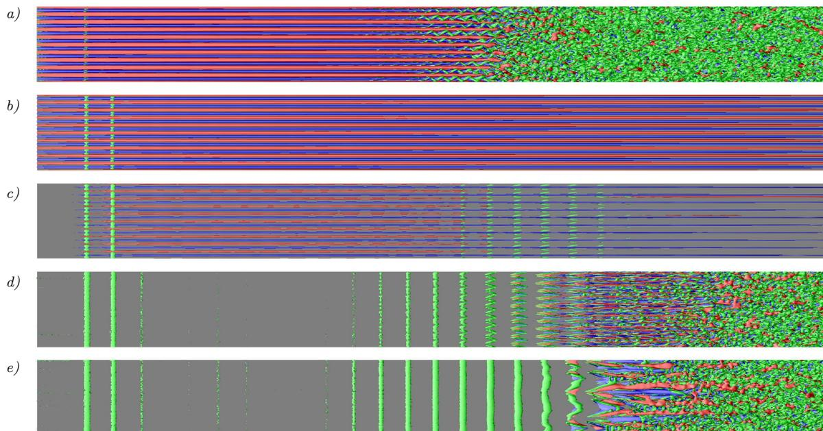
Figure 10: Top view of the three-dimensional flow structures for streaks A, C, D, F, N (uncontrolled), from *a*) to *e*). Green isocontours represent the  $\lambda_2 = -0.00008$  vortex-identification criterion, red and blue isocontours are positive and negative disturbance velocity  $u' = \pm 0.07$ , respectively. Flow from left to right.
