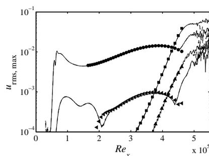
Figure 4: Evolution of various Fourier modes for H-type (subharmonic) transition (Herbert, 1993). — current LES; symbols: PSE. • mode  $(\omega_0, 0)$ , ■  $(\omega_0/2, \beta_{\text{crit}})$ , ◀  $(2\omega_0, 0)$ , ▲  $(3\omega_0/2, \beta_{\text{crit}})$ .
