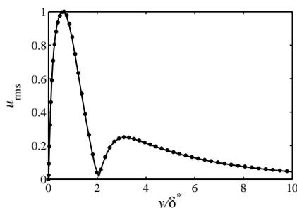
Figure 2: Comparison of TS-waves obtained by LES with LST.  $u_{\text{rms}}$  at  $Re_x = 216000$ , — LES, • LST.
