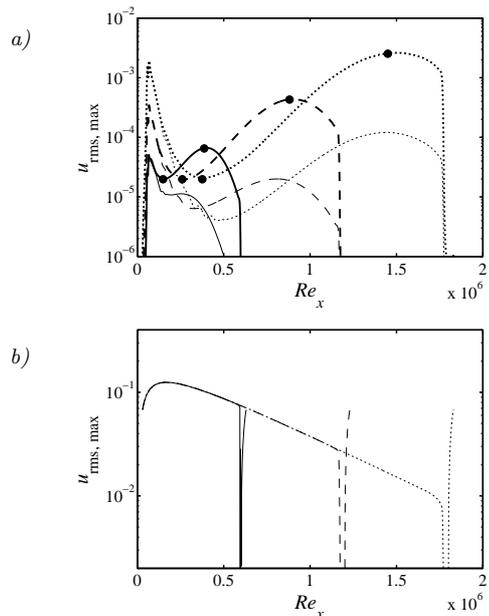
Figure 6: Streak C and 2D TS-waves of different amplitude and frequency. —  $F = 120$ ,  $A_{TS} = 2.575 \cdot 10^{-5}$ , ---  $F = 70$ ,  $A_{TS} = 1.692 \cdot 10^{-4}$ , .....  $F = 50$ ,  $A_{TS} = 1.000 \cdot 10^{-3}$ . *a)* Mode  $(\omega_0, 0)$ , thick lines are only TS-waves, thin lines controlled with streak C. • position of branch I and II according to LST. *b)* Streak amplitude  $u_{rms,max}$ .
