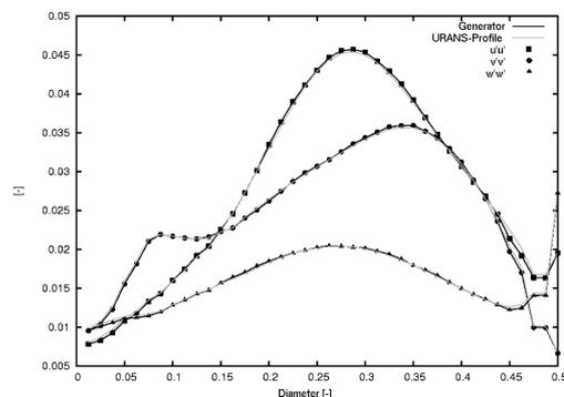
Figure 3: Reynolds stress components from generated fluctuations and target profiles.
