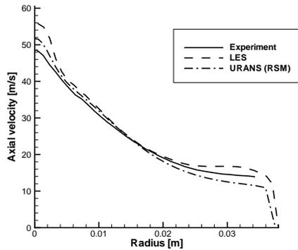
Figure 7: Axial velocity before vortex breakdown.
