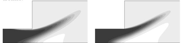
Figure 10: Temperature contours with (right) and without (left) quenching model applied.
