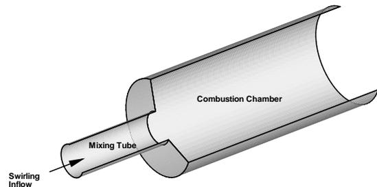
Figure 1: Configuration of the swirl burner.
