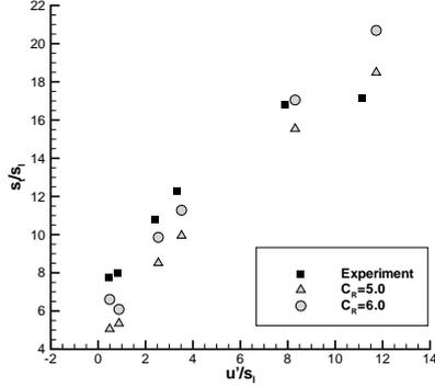
Figure 4: Ratio of turbulent to laminar burning velocity plotted over fluctuations to laminar burning velocity at two different values for the LV-model constant  $C_R$ .
