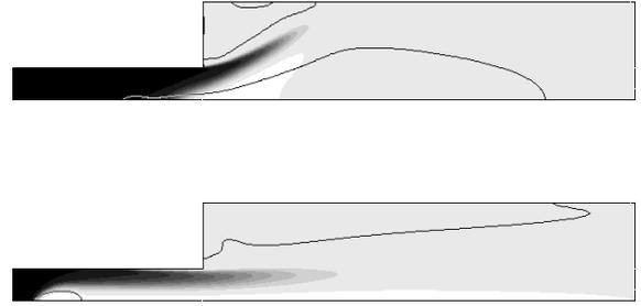
Figure 9: Contours of the temperature, stable flame and flashback state. Recirculation zone marked by an  $u_{ax} = 0$  isoline.
