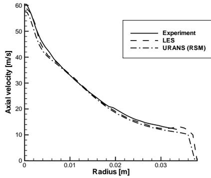
Figure 6: Axial velocity close to inlet.
