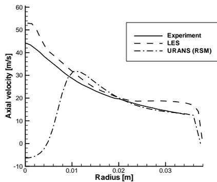
Figure 8: Axial velocity behind vortex breakdown in URANS.
