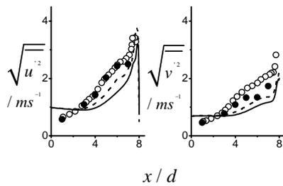
Fig. 5: Fluctuating velocities along the stagnation line ( $\circ$  data,  $\bullet$  cross-referenced data, — RANS, - - - - - LES).
