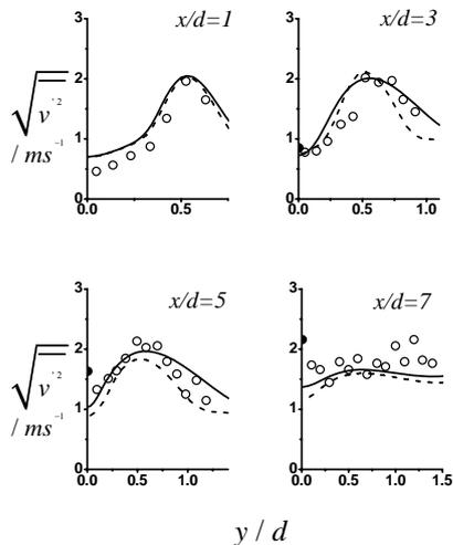
Fig. 3: Parallel-to-wall fluctuating velocities at various distances from the surface ( $\circ$  data,  $\bullet$  cross-referenced data, — RANS, - - - - LES).
