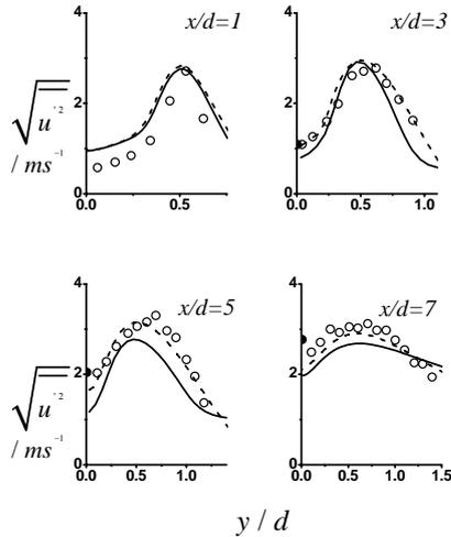
Fig. 2: Normal-to-wall fluctuating velocities at various distances from the surface ( $\circ$  data,  $\bullet$  cross-referenced data, — RANS, - - - - LES).
