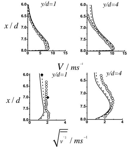
Fig. 6: Parallel-to-wall mean and fluctuating velocities in the wall jet region ( $\circ$  data,  $\bullet$  cross-referenced data, — RANS, - - - - - LES).
