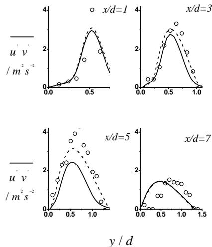
Fig. 4: Shear stress at various distances from the surface ( $\circ$  data, — RANS, - - - - LES).
