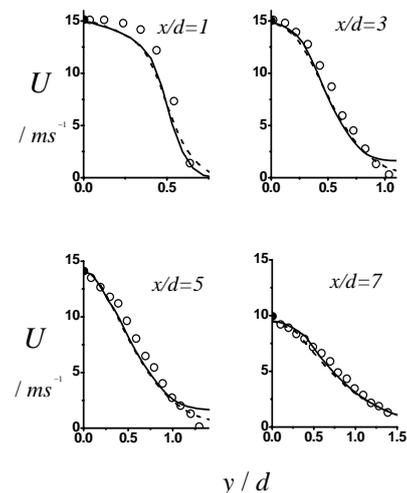
Fig. 1: Normal-to-wall mean velocities at various distances from the surface ( $\circ$  data,  $\bullet$  cross-referenced data, — RANS, - - - - LES).
