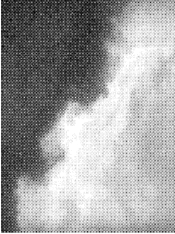
Figure 3: Experimental quantitative image of a gas-phase turbulent separated shear layer at Re \sim 10^6 , M \sim 0.9 , and Sc \sim 1 , at a pressure of \sim 3 atm, recorded in the UC Irvine Aero-Optics Flow Facility.
