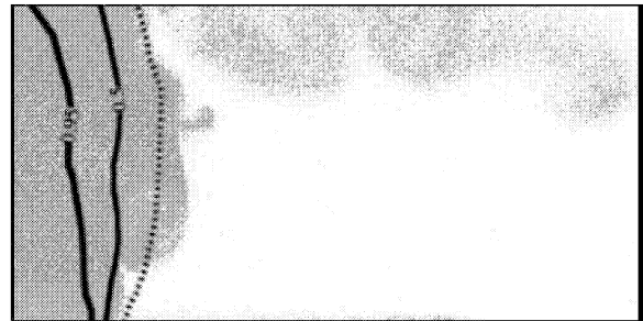
Figure 5: Acetone concentration image, together with iso surfaces taken from the DNS (95%, 50%, 20%) representing the concentration. A cloud of the heavy acetone-mixture stagnates at the upper right edge of the picture.
