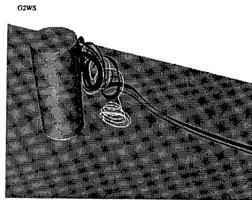
Figure 12: Visualization of the vortex structure behind the cylinder (run G2WS).
