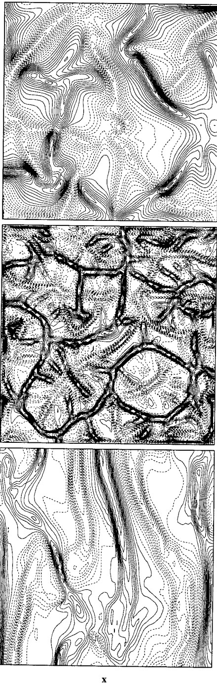
Figure 8: Vertical velocity ( W ) distribution in the central horizontal plane ( z/D=0.5 ), Ra=10^7 , Pr=0.025 : first- Ha=0 , no magnetic field; second- Ha=200 , transversal magnetic field ( B||z ); third- Ha=200 , longitudinal magnetic field ( B||y ).
