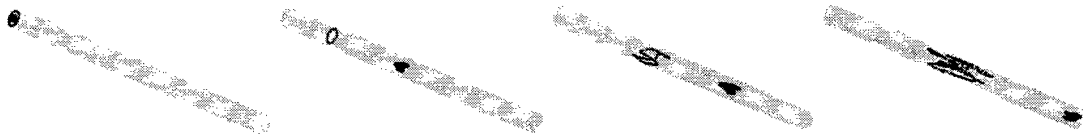
Figure 6: Transport of marker particle rings through the elliptic stenosis. The thick, solid ring and the thin ring correspond to \frac{1}{4} and \frac{3}{4} the main vessel diameter, respectively.
