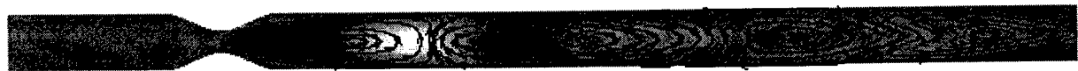
Figure 8: Countours of vertical velocity and streamlines of dominant two-dimensional Floquet mode for periodic flow with \alpha = 4 and Re = 150
