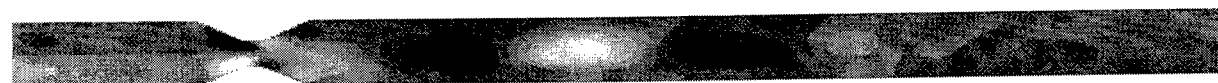
Figure 9: Vertical velocity distribution at 11/16 cycle for periodic flow with \alpha = 4 and Re = 150
